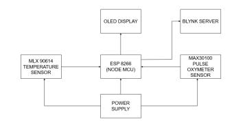
Fig. 2. Block Diagram for Biotelemetry
